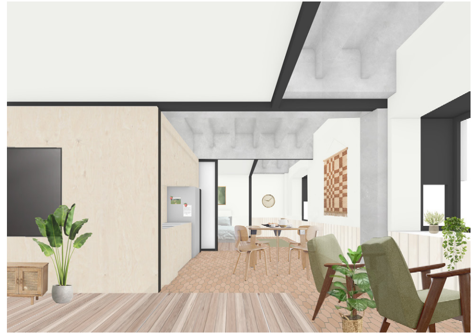
UNITS (H): "Hidden sliding screen doors within a core, paneled as a large piece of pine furniture, can be extended to close off spaces...New window boxes transform existing concrete sunshades into extensions of the interior."
