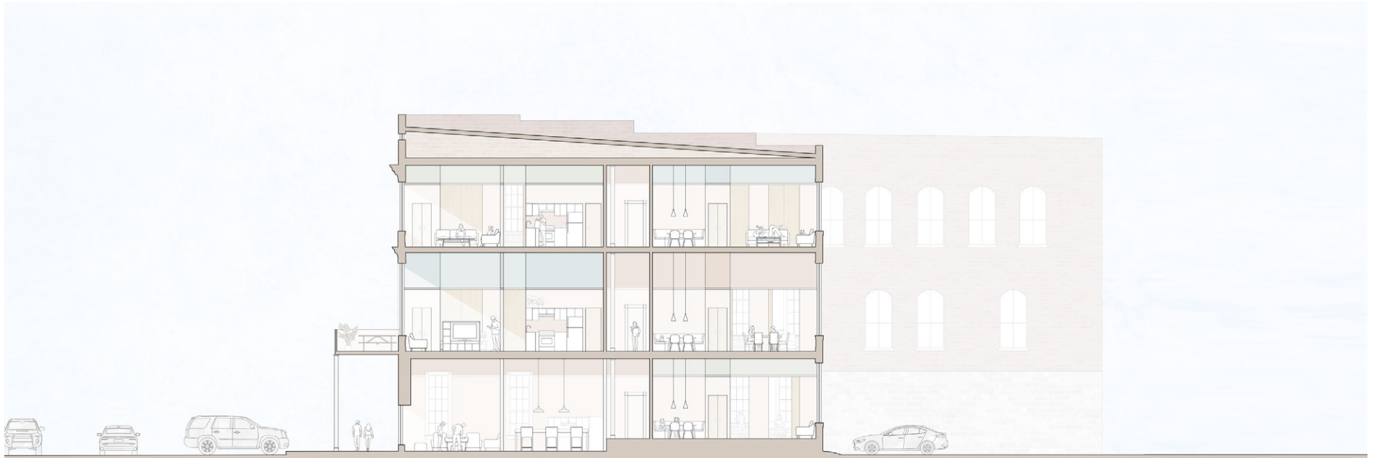
SECTION: "Each bedroom and living area has at least one 12-foot tall existing window...Additionally, each unit has interpreted an historical double parlor to allow for natural light from the living area to reach the kitchen and dining area."
