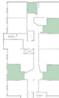
OPTION 2: TERRACES CIRCULATION: 1620 sq ft SHARED / EXTERIOR SPACE: 1970 sq ft TOTAL COMMUNAL SPACE: 3590 sq ft
