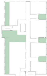
OPTION 1: SUNROOMS CIRCULATION: 1650 sq ft SHARED / EXTERIOR SPACE: 1930 sq ft TOTAL COMMUNAL SPACE: 3580 sq ft
