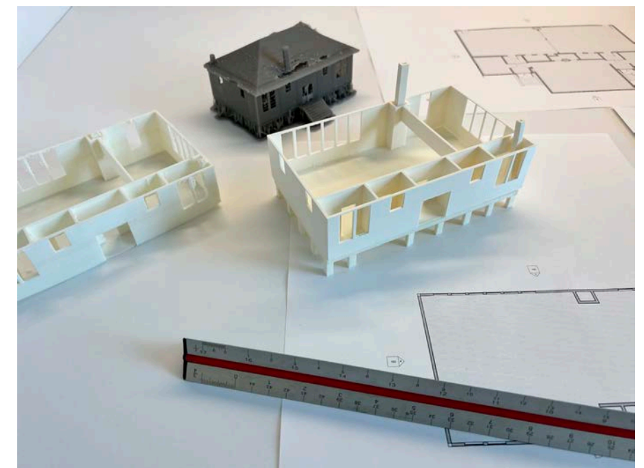
Screen shot of the LiDAR Pointcloud of the interior of Tankersley Rosenwald School (above) In process 3D Printed models that translate the digital point clouds to physically printed models (below)
