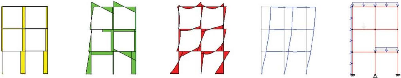
Working backward - predicting configuration and applied loading from force diagrams.
