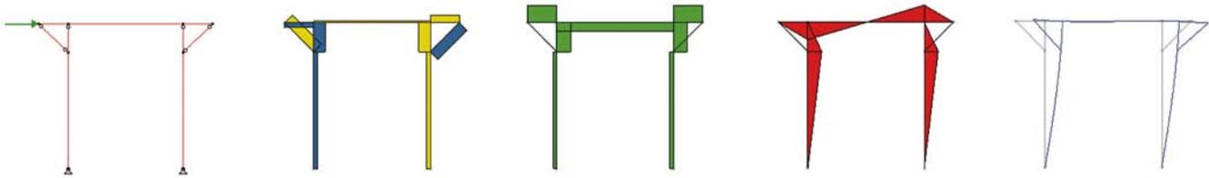
Working forward - predicting force diagrams from configuration and applied loading
